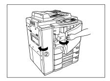
**2** Remove the used toner bag from the copier in the direction of the arrow.
